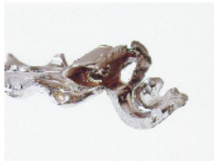
**15** Check that the solder has flowed completely around the threaded cap. If a solder model was used, remove investment residue from the threaded cap after soldering with an ultrasonic cleaner. Prepare the solder joint and then insert the patrix in the threaded cap.
