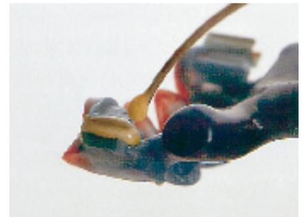
**4** After mixing the required amount of investment (according to the size of casting ring), hold the rubber base vertically on the vibrator and use a probe to ensure the investment flows into the attachment channel. (Do not press in!)
