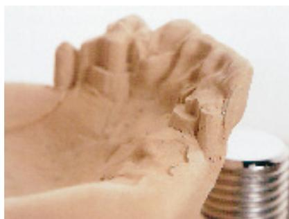
**10** Duplicate according to the instructions. The threaded cap is clearly defined on the investment model after removal of the duplicating material.
