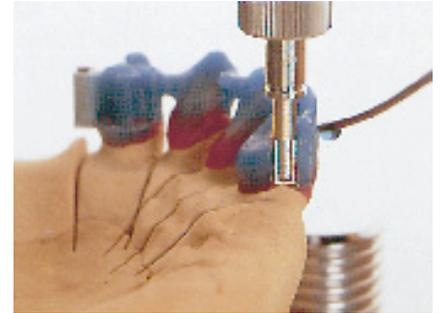
**2** Then create sufficient space for the matrix. Place the matrix on the crown wall or in the recess and wax it in position.
