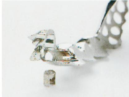
**25** Sandblast the threaded cap and the threaded cap recess in the CrCo framework with 250  $\mu\text{m}$  corundum at approx. 5 bar pressure. Remove the block out wax with a steam cleaner.
