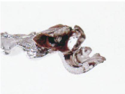
**14** Apply antiflux to the threads and the inner surfaces of the threaded cap. Apply flux to the surfaces to be soldered. Ensure that the flux has flowed completely round the threaded cap. Solder in the usual way.
