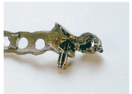
**33** Check that the solder has flowed completely round the attachment matrix. Prepare the solder joint and polish the CrCo framework. Assemble the spring, bolt and press lock and check that the attachment functions properly.
