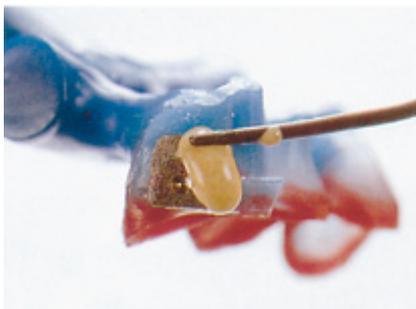
**5** Mix the required amount of investment. Hold the rubber base vertically on the vibrator. Use a probe to ensure the investment flows around the attachment channel and lock recess.
