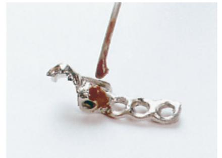
**30** Apply flux to the outer surfaces of the matrix and to the CrCo framework.
