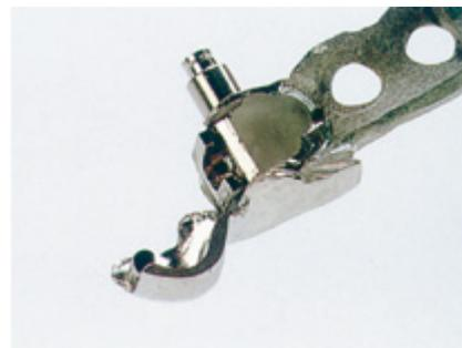
**24** After the DuroBond has cured, lift the CrCo framework from the crowns and remove any excess composite. Check that the lock functions properly.
