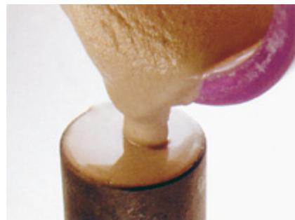
**6** Place the casting ring on the base and fill the mould with the investment.
