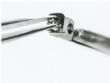
**17** Remove the lock bolt and compression spring.
