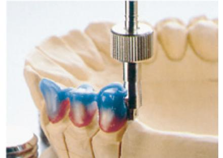
2 Determine the path of insertion and place the patrix temporarily on the crown wall with the paralleling mandrel No. 640. Shorten the patrix if required. Place the patrix in position and mark the outline on the crown. Then create sufficient space for the patrix.
