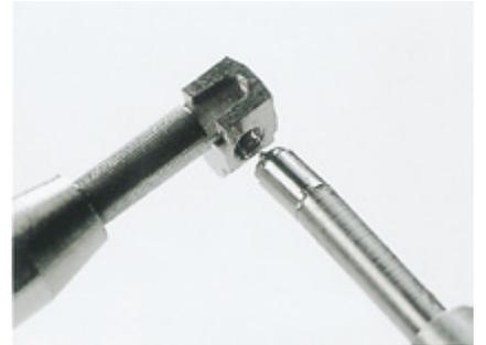
**16** Unscrew the lock from the matrix. Hold the lock bolt in position with instrument No. 642 to prevent it springing out spontaneously.
